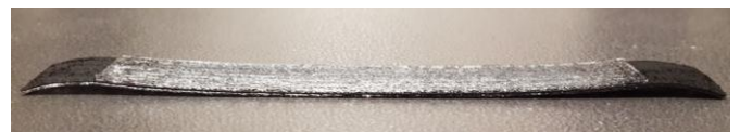
Figure 1. The 3D printed sensor. PLA-G is sandwiched between two layers of TPU. At the two ends, PLA-G is designed to be exposed to facilitate wire bonding.
