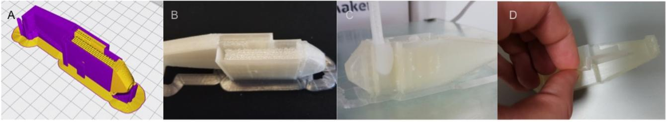
Fig. 2: Fabrication process of a soft actuator. (A) Slicer settings with build-material in yellow and resolvable material in purple. (B) Finished print of the shell, the rigid components and the structure for mechanical bonding. (C) Casting the two silicone components. (D) Removing or dissolving the resolvable material.
