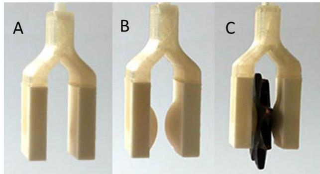
Fig. 1: Multi-material soft pneumatic gripper having a rigid 3D-printed body connected with two silicone parts through a mechanical bonding. Upon pressurization, the zero-thickness chamber between the silicone and rigid body expands. From left to right: the gripper in rest shape (A), the inflated gripper (B), and the status of grasping a chocolate (C).
