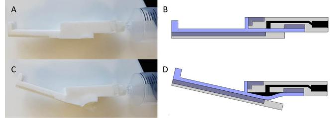
Fig. 3: A single gripper finger mechanism before (A) and after (C) pressurization. The zero-thickness chamber is inflated through the internal air channels and pushes the rigid element outwards to realize a grasping function. Cross-sectional views of the gripper's mechanism for both states are given in (B) and (D). Rigid bodies are indicated in gray, air channels in black, silicone parts in blue and bonding parts in purple.
