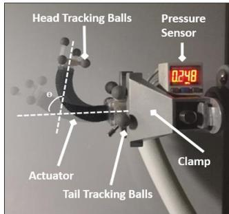
FIG. 3. Testing set-up and experimental results for actuator
