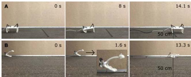
Fig. 3. Locomotion robots based on SOVA. Time sequence of locomotion robots (A) Walking robot (B) Hopping robot – Gongaroo
