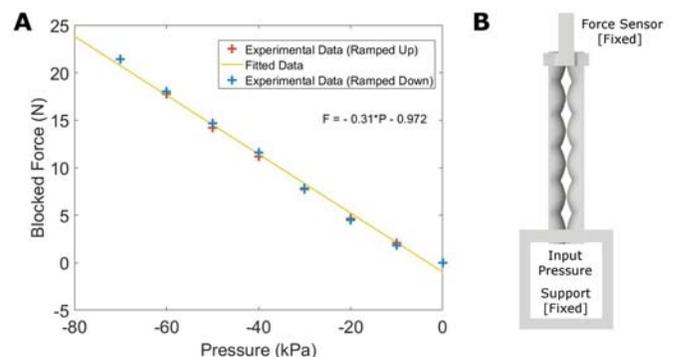
Fig. 2. Blocked force of SOVA. (A) Blocked force curve (B) Blocked force experimental setup.
