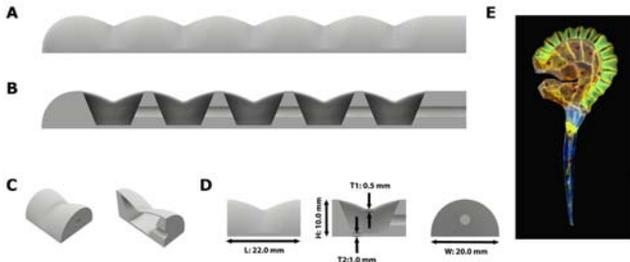
Fig. 1. Soft vacuum actuators (SOVA). (A) Soft actuator computer aided design (CAD) model (B) Section view of soft actuator CAD model. Pneumatic hinges are connected through a 3.0 mm diameter hole. (C) Pneumatic hinge CAD model (D) Pneumatic hinge dimensions. L: Hinge Length, T1: Hinge Wall Thickness, T2: Hinge Base Thickness, W: Hinge Width (E) Annulus of fern sporangia (Used with permission) (4).
