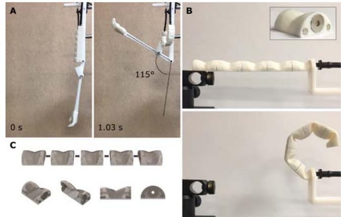
Fig. 4. Soft artificial muscles and modular actuators based on SOVA. (A) Soft artificial muscle – elbow angular stroke (B) Bending behavior of modular SOVA (Inset: 3D printed soft pneumatic hinge with magnets) (C) 3D computer aided design (CAD) model along with a single hinge model for the modular actuator
