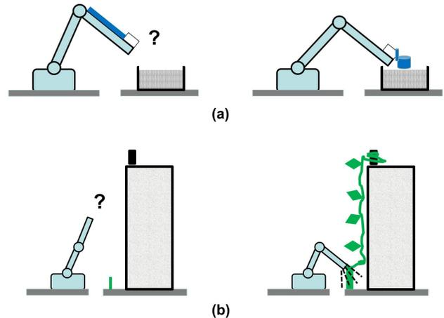
Fig. 1. Robots with EPs are able to extend their task handling capabilities. (a) An example where a robot (arm) makes an artefact of a scoop (in blue) for getting liquid from a container. (b) Another example where the robot exploits a living plant (in green) to reach a target (in black) beyond the initial reaching range of the robot.
