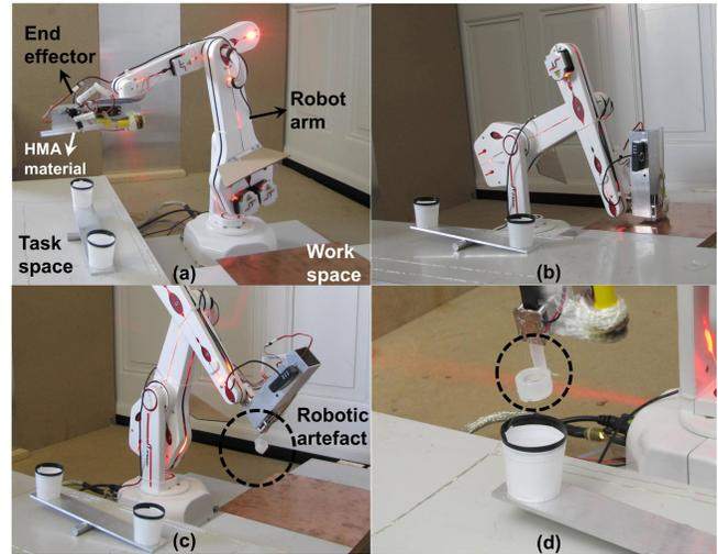
Fig. 2. A case study of a task exemplified as in Fig. 1a. (a) A robot identifies task requirements. (b) The robot makes a scoop artefact as EP. (c) EP is shown in a dashed circle. (d) The robot uses the scoop to get water from one container to the other. The material used by the robot to make the artefact is thermoplastic adhesive. Photo courtesy L. Brodbeck.
