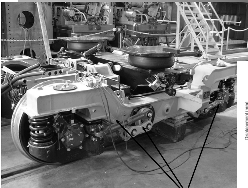
Fig. 15. Experimental roller rig tests—lateral wheel-rail deflection.
